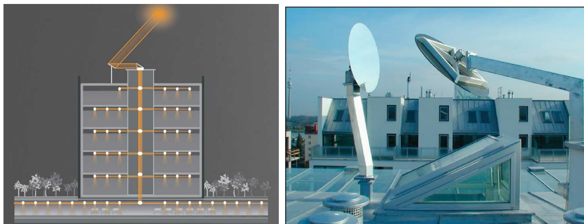
Left: Heliostat lighting, principle; right Heliostat collector M. Mayhoub, Fifty years of building core sunlighting systems—Eight lessons learned, Solar Energy 184 (2019) 440-453.
